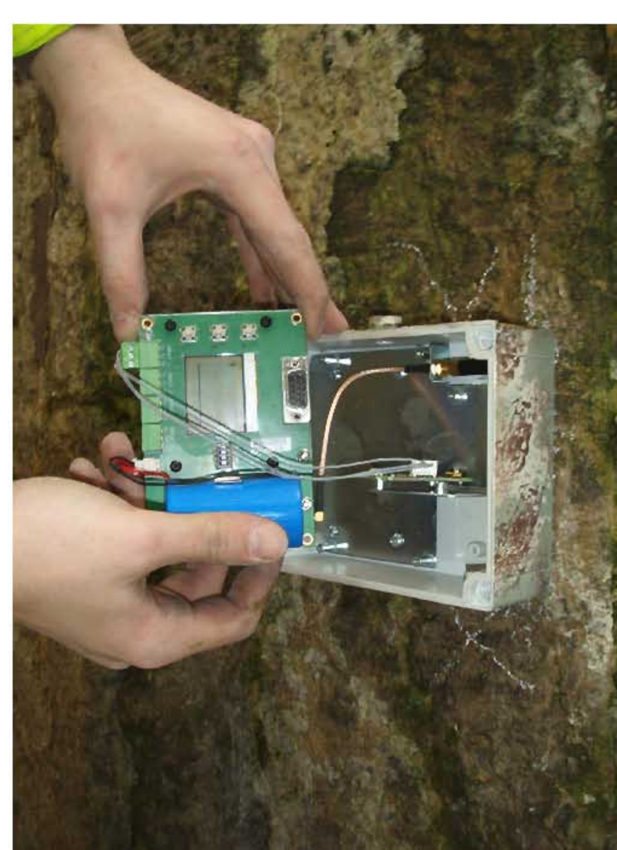
One of the electronic devices used to monitor movement of structure
