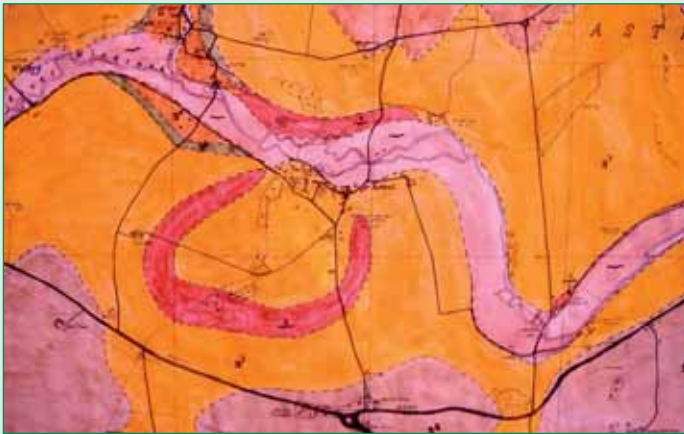
The geology of Asthall showing a u-shaped patch of gravel that was left as the course of river changed after the last ice-age
